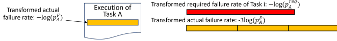
Fig. 1: Example of task re-executions to satisfy the failure rate constraint of Task A, which requires executing the task at least 3 times; the failure rates are transformed with a negated logarithm function so that the failure rate after re-execution can be visually represented as a summation; the relationship between the bars is equivalent to p_A^{req} \geq p_A^{F^3} .
